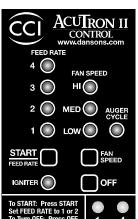
through the FEED RATE touch pad, to vary your heat output from Low to High. The room air fan can be manually adjusted through the FAN SPEED to run faster or slower to correspond to the amount of heat being produced. The room air fan is also on a limit switch, controlled to run on high when the stove reaches higher temperatures and then resume the speed you had selected once it cools to a lower temperature.
